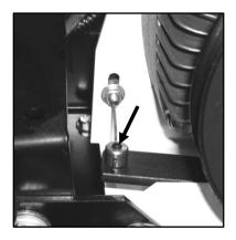
Figure 30: Pivot Pin and Setscrew
